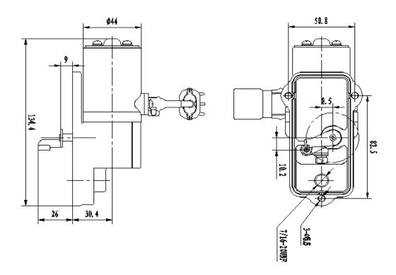
The outline and installing size of the A100C-W electromagnetic actuator
